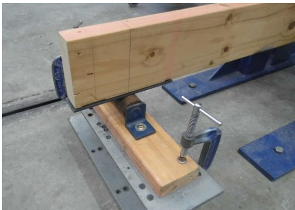
Photograph 3. Support at end of long leg.
