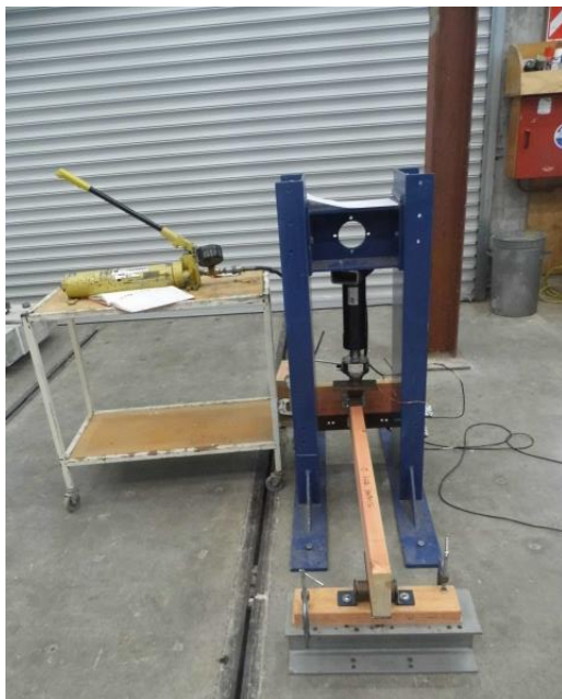
Photograph 2. Test set up for Shear 1 configuration
