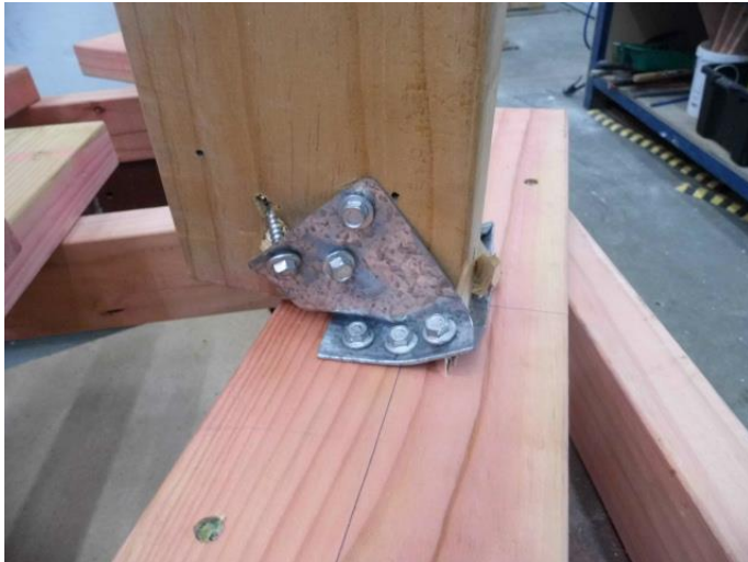
Photograph 8. Failure by distortion of the bracket and screw withdrawal
