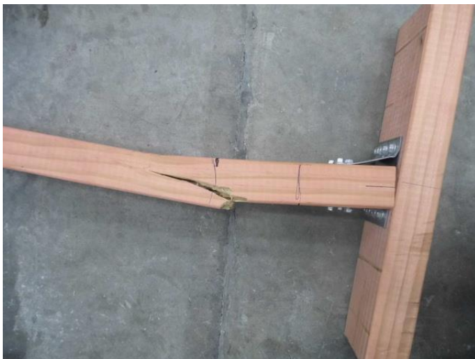
Photograph 7. Failure by timber fracture under the load point (initial test)
